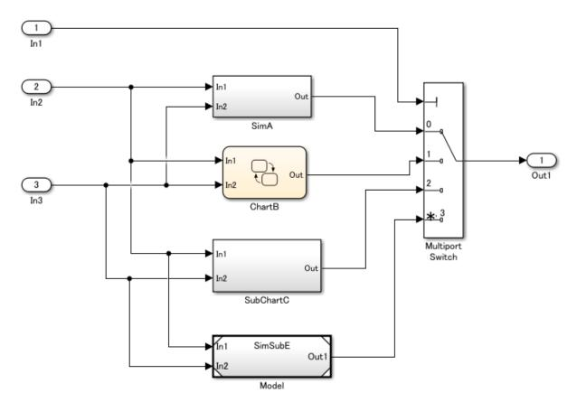
For example, the model model\_ref contains the Model block SimSubE.
