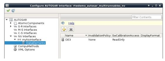
4 In the left-hand pane of the Configure AUTOSAR Interface dialog box, under AUTOSAR, select AtomicComponents. Expand AtomicComponents and select an AUTOSAR component. Expand the component.
