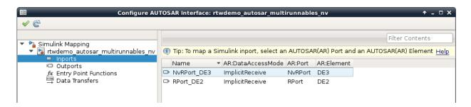
To programmatically configure AUTOSAR NV data communication elements, use the AUTOSAR property and mapping functions. For example, the following MATLAB code
