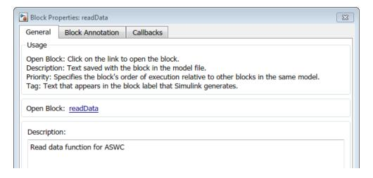
When you export arxml for the model, the generated runnable description contains the Simulink description text.
