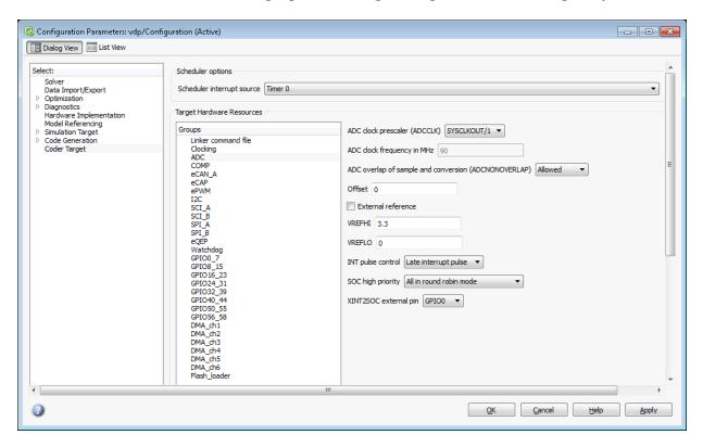
This Coder Target pane has a the same name as the Code Generation > Coder Target sub-pane that appears when the **System target file** parameter is idelink\_ert.tlc or idelink\_grt.tlc.
