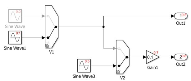
For example, the model VariantMergeReuse contains two Variant Source blocks.
