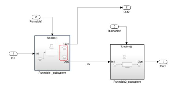
Beginning in R2014b, AUTOSAR code generation supports branching outside the runnable. This modeling pattern can potentially generate more efficient C code, for example, with fewer global variables and fewer block I/O buffers.
