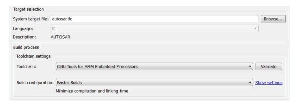
Other targets that support toolchain controls include the ERT targets ert.tlc and ert shrlib.tlc.
