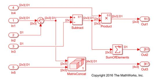
In R2017a, the code generator can reorder the block execution order so that the Matrix Concatenate block executes before the Subtract block and the Sum of Elements block executes before the Product block. Reordering block operations eliminates the two temporary arrays, the two variables, and their associated data copies from the generated code. The blocks can use the same variable for the input and output.
